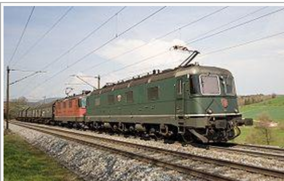
Re 620 and Re 4/4 II or III leading a freight train on the northern Bözberg incline
